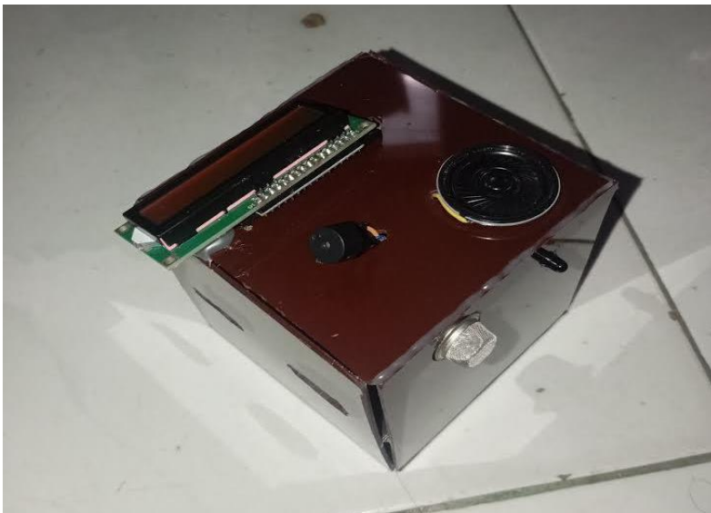
Figure 9. Actual Photo of the Enhanced Smoke Detector
