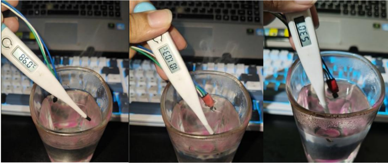
Figure 11. Experimental setup for the accuracy testing of the HeatEye prototype
