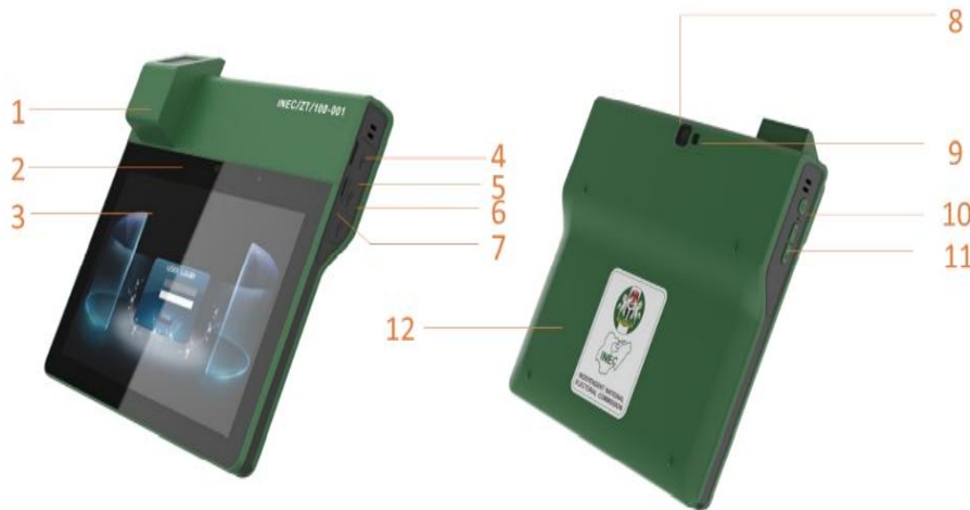
Figure 1.0: The numerically labelled features of the BVAS/IVED tablet (Election Technologies Manual, 2022)
