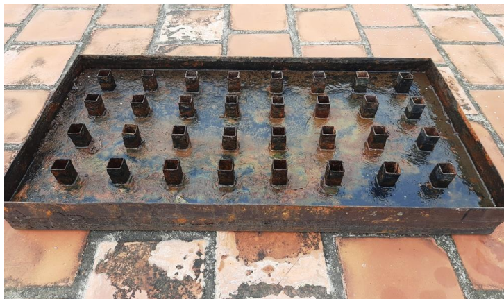
Fig. 1. Photograph of the basin liner fitted with 32 square hollow tubular fins.
