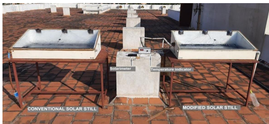
Fig. 2. Photograph of the experimental setup showing the conventional and modified stills with the solarimeter and temperature indicator.
