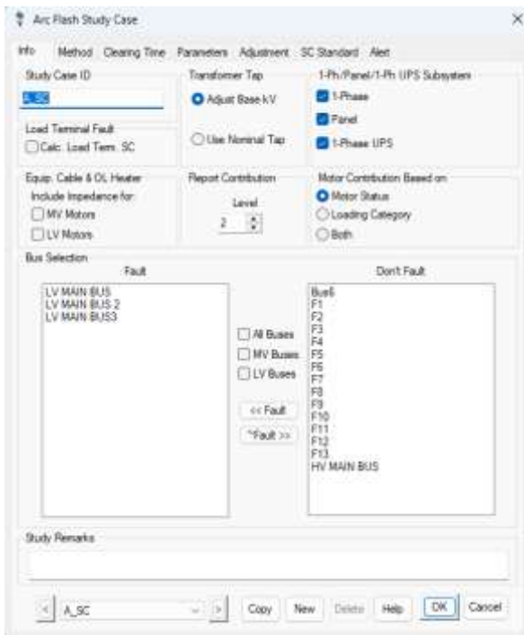
Figure 3 Arc Flash Study, defining faulted buses
