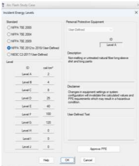
Figure 5 Incident Energy levels for PPE consideration
