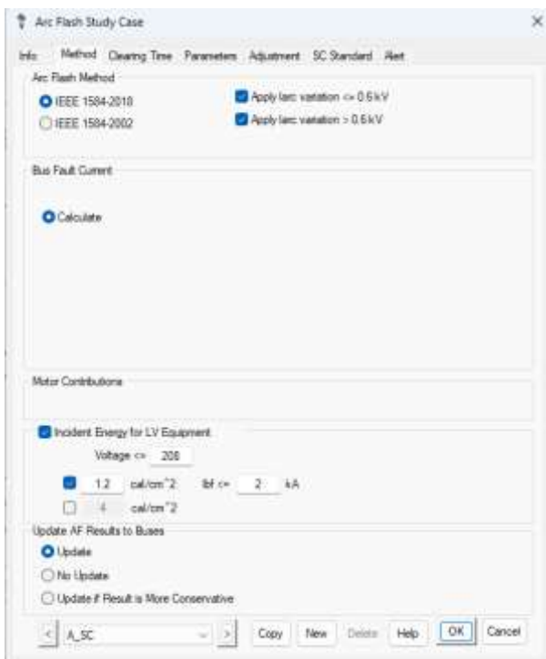
Figure 4 Defining methodology for arc flash study case
