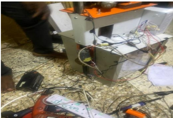
Figure 18: Image of the Opening and Closing Motor Mounted at the Rear of the Waste Bin
