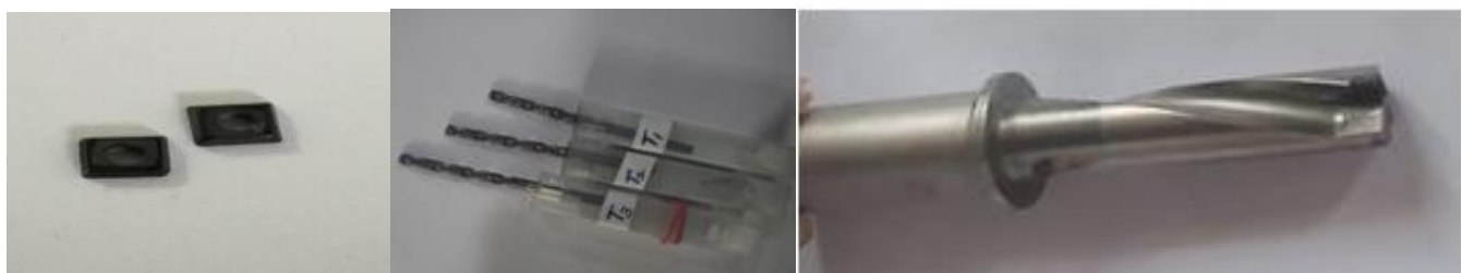
Figure 2. (a) Plain carbide inserts (b) Tungsten Carbide twist drill, & (c) U-drill
