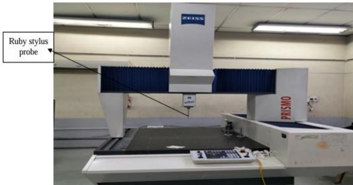
Figure 4. Zeiss Prisma Co-ordinate measuring machine (CMM)
