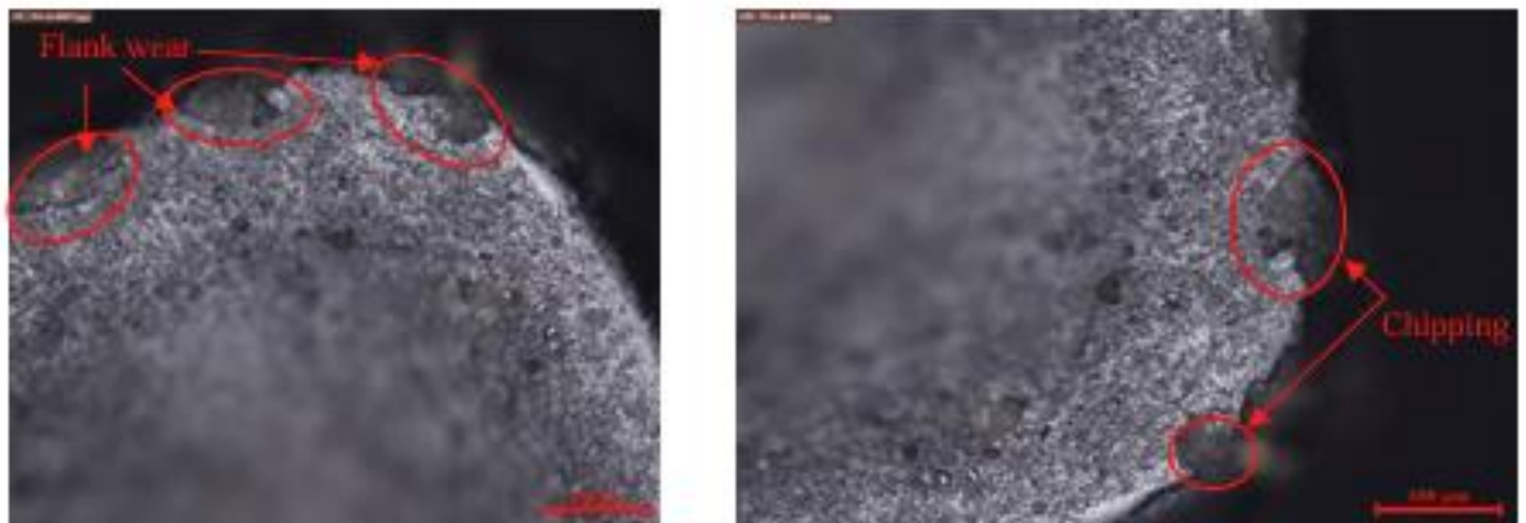
Figure .5 Microscopic images of Plain carbide drill insert after machining
