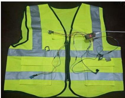
Figure 8. Preliminary SmartVest Prototype Integration and Sensor Configuration
