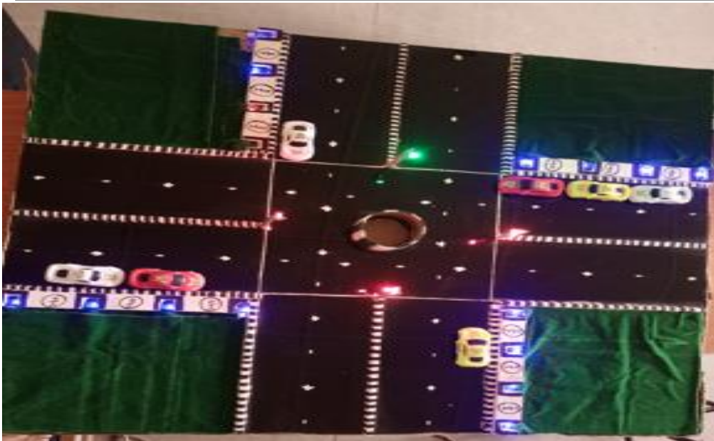
Figure 8: Testing the prototype for identifying and giving priority to road with highest traffic volume
