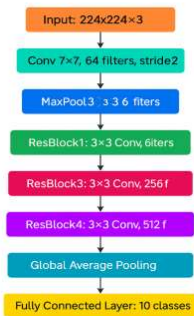
Figure 1: ResNet-18 architecture pipeline for CIFAR-10, with 224×224 input, residual blocks, global average pooling, and a 10-class linear output head.
