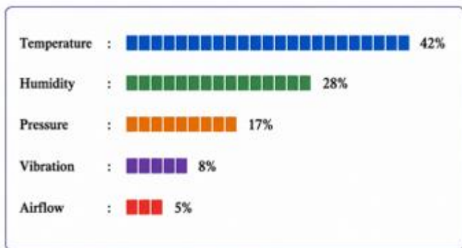
Figure 3. The uncertainty of calibration that can be attributed to the environment.
