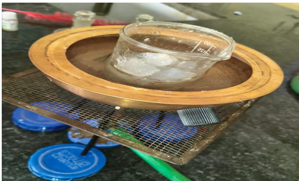
Figure 4: Melting of Soap Base on Water Bath
