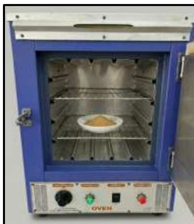
Figure 14: Drying the granules in hot air oven
