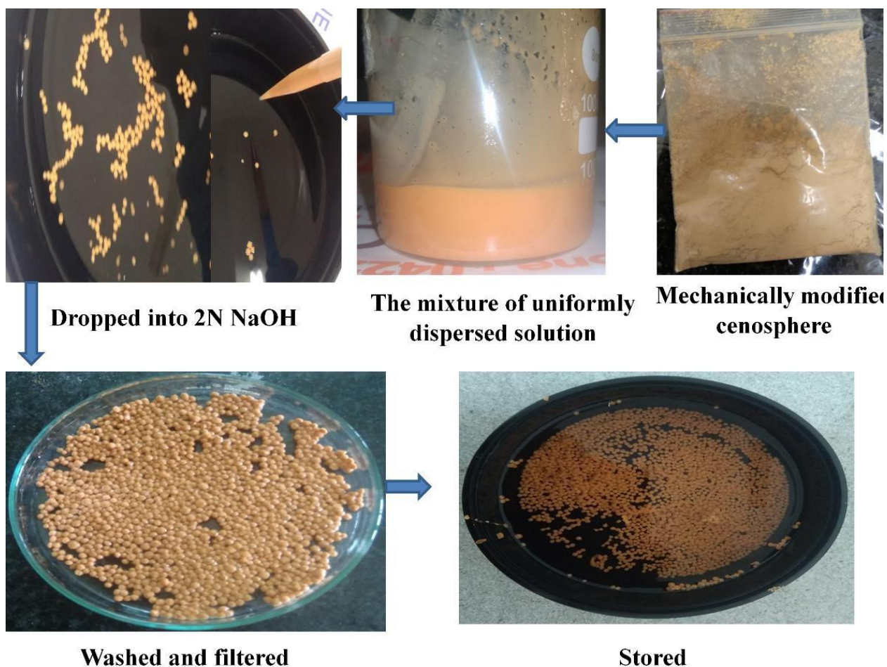
Figure 1 Method and procedure for TiO 2 coated cenosphere.
