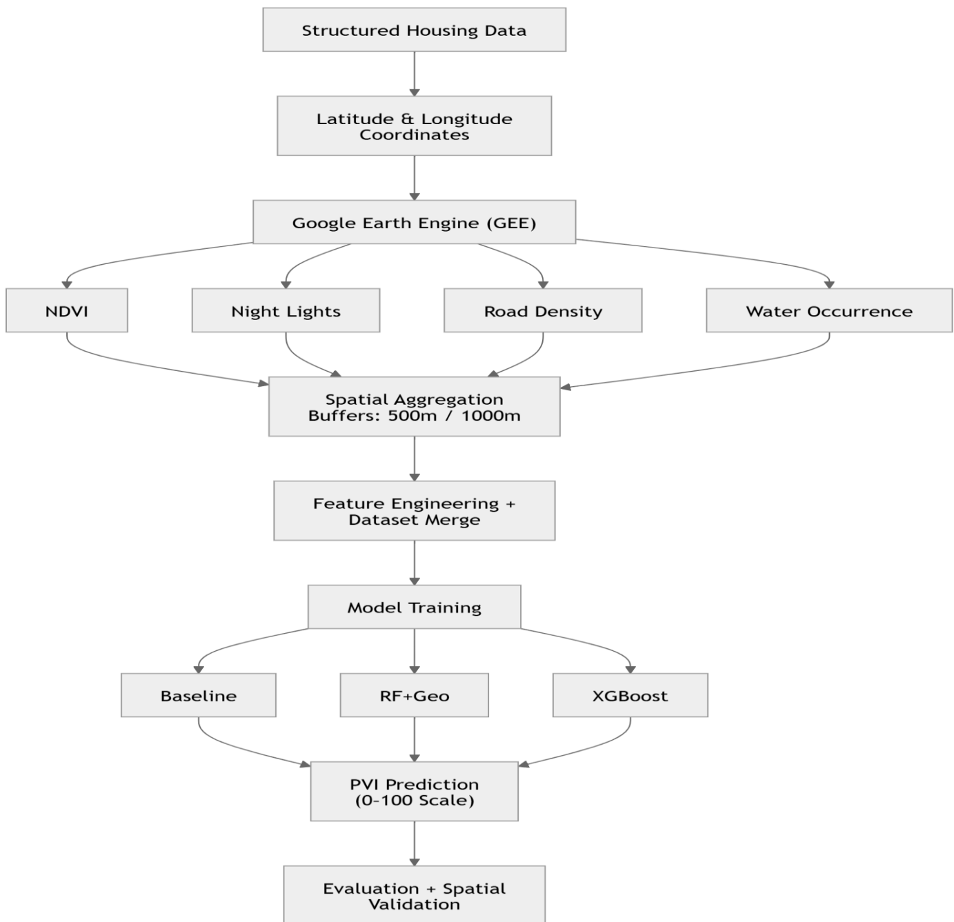
Figure 1: Geospatial property valuation pipeline integrating structured data, GEE-derived features, and machine learning models.
