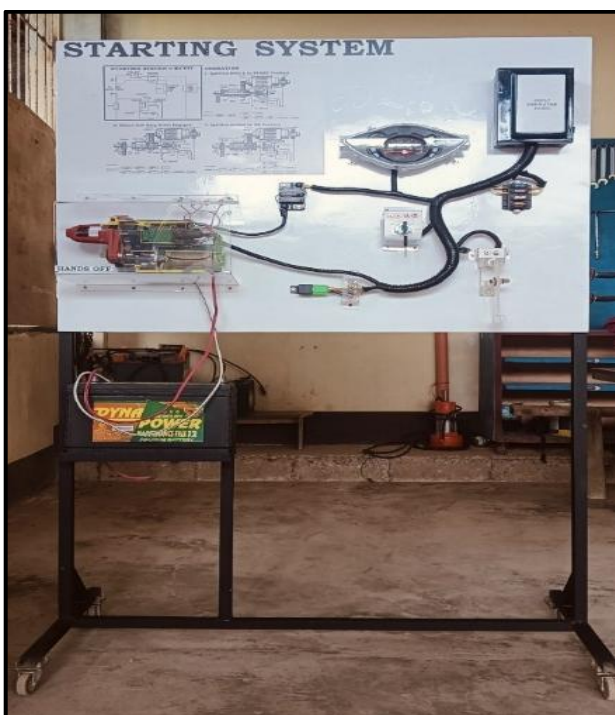
Figure 2. Actual Gear Reduction Starting System Simulator
