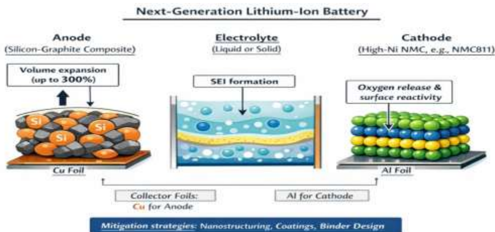
Figure 5 Schematic showing the components of a next-generation lithium-ion battery with silicon-composite anode and high-nickel cathode. Annotate with key challenges.
