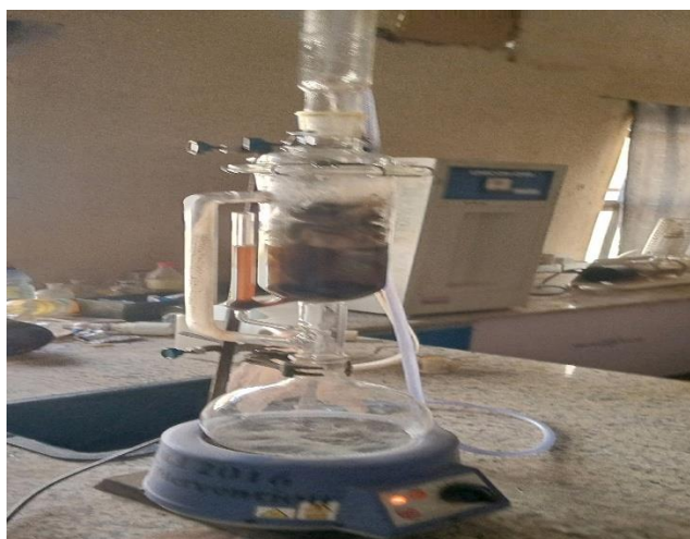
Figure 4 Picture of Soxhlet Extractor used to extract CNSO
