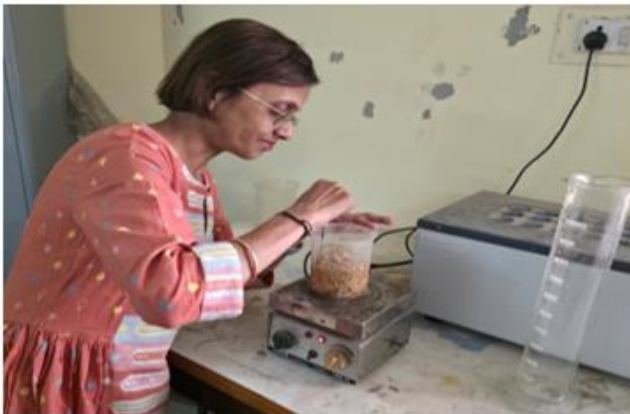
Picture 3: Chemical Activation Process with Phosphoric Acid
