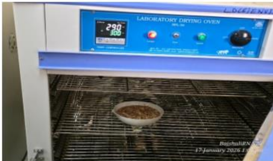
Picture 4: Thermal treatment at 300 degree C
