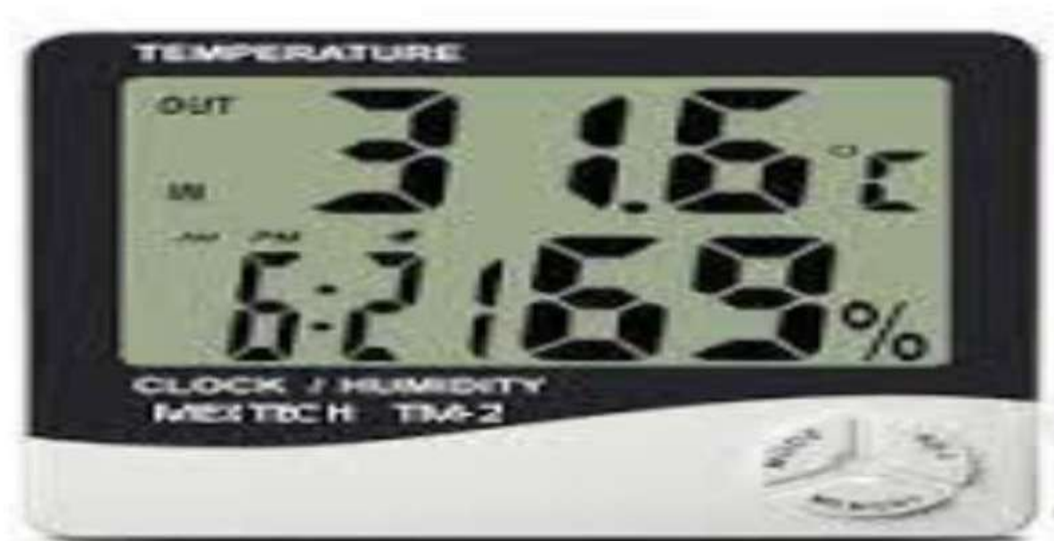
Fig. 2.2: Digital thermo-hygrometer used to record humidity of the air and temperature of the air
