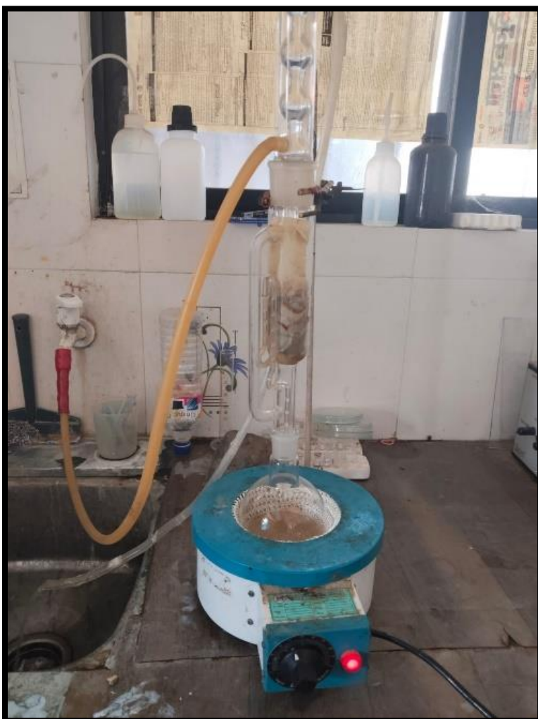
Ethanollic Extraction Using Soxhlet Apparatus Ashwagandha ( Withania somnifera ) & Shilajit
