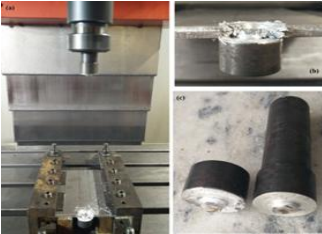
Figure 14: Experiment-2, broken tool-2, (a) experiment setup, (b) view of bottom shoulder, (c) view of broken parts of tool-2.
