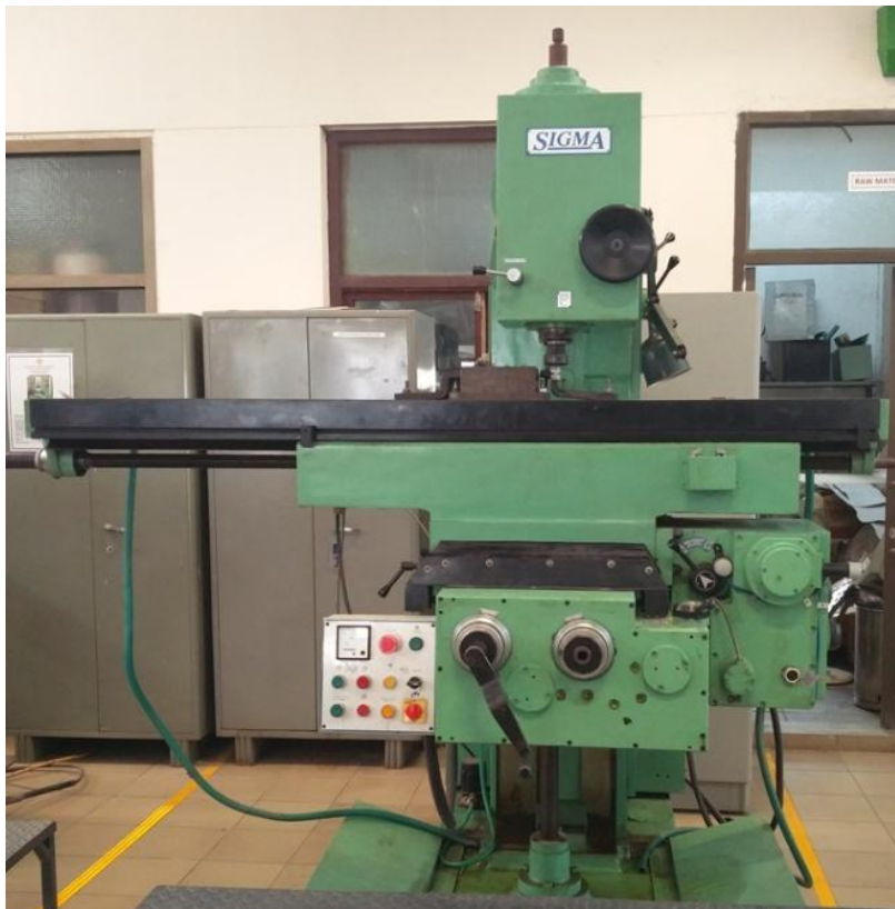
Figure 15: Heavy duty vertical milling machine used for FSW
