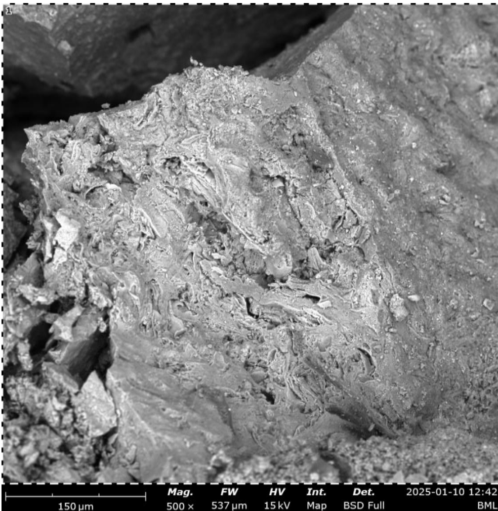
Figure 4: SEM Result of ZnO Nanoparticle Synthesized Using Leaf Extract
