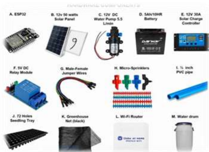
Figure 2. Hardware Components of Solar-Powered Automated Sprinkler Irrigation System
