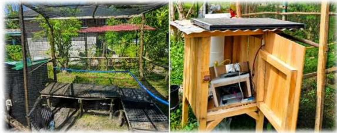
Figure 10. Hardware Setup of the Solar-Powered Automated Sprinkler Irrigation System
