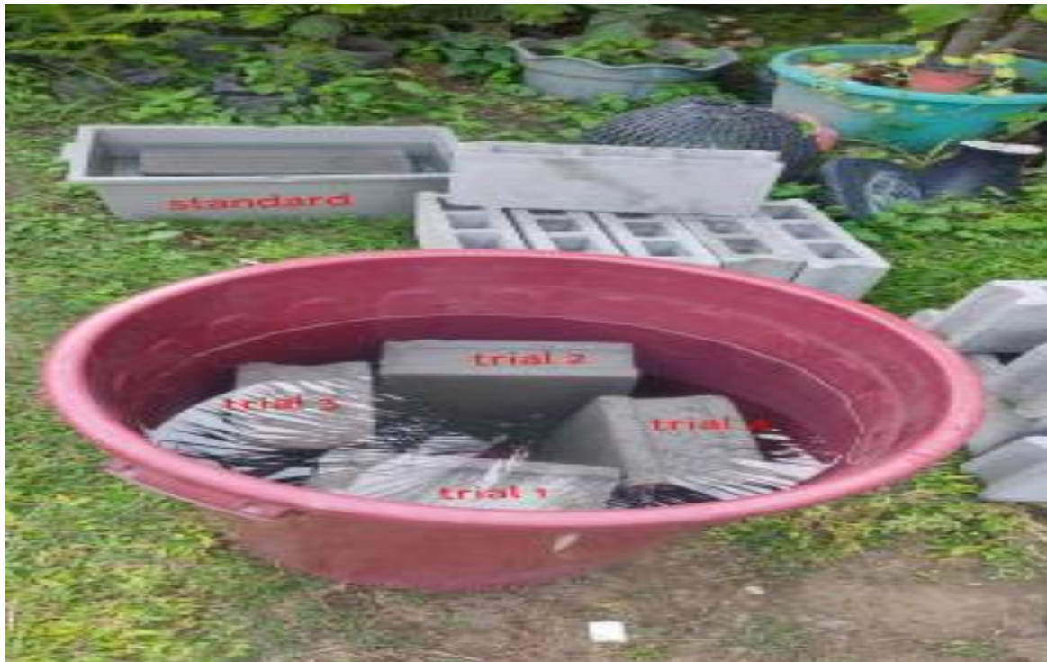
Figure 3. Water Absorption Testing
