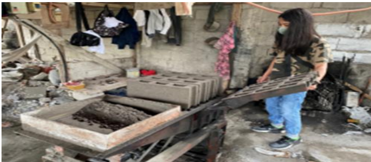
Figure 1. Production of Sample Hollow Blocks
