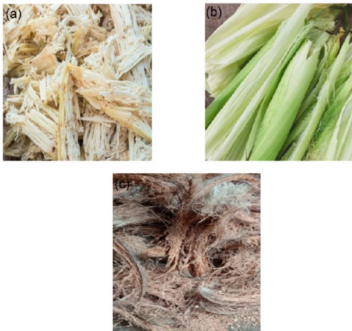
Fig 1. Agricultural waste (a) sugarcane bagasse (b) corn husk and (c) coconut sheath
