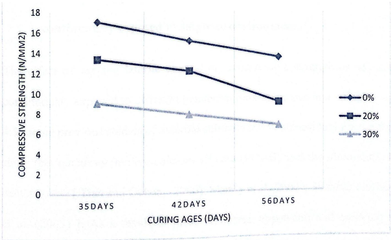
Figure 2 Residual compressive strength of superplasticized laterized concrete exposed to 1% magnesium sulphate concentrate solution.
