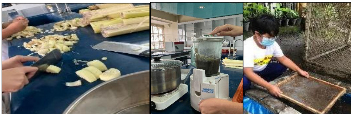
Figure 2. Production of MuSk Fibers Using Banana Pseudo Stem
