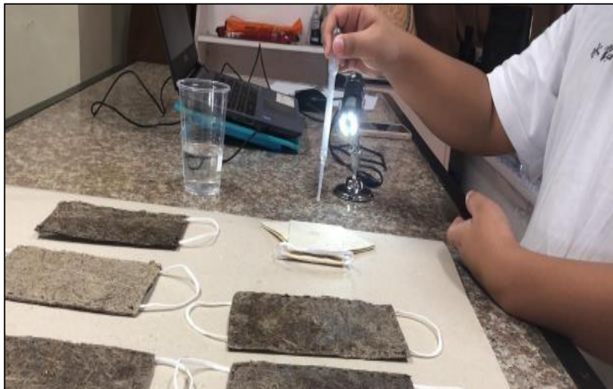
Figure 5. Testing the Hydrophobicity Property of MuSk Surface
