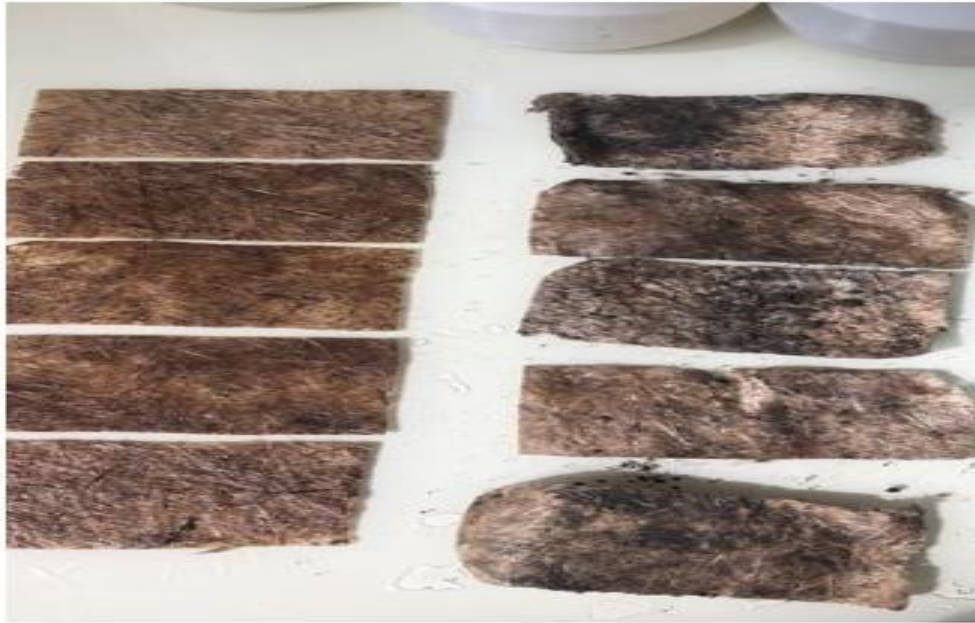
Figure 7. Testing the Biodegradability of the MuSk Fiber
