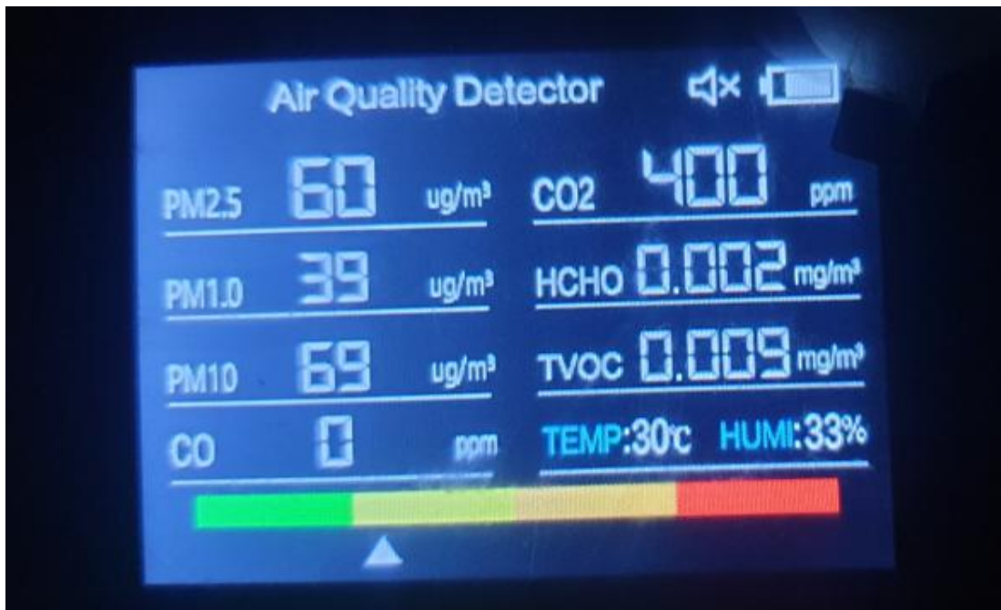
Figure 10. 9-in-1 air quality detector readings under clean-air conditions
