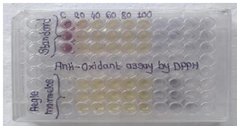
Fig. 3.5 - 96 wells ELISA plate showing colour change from purple to yellow at different concentrations
