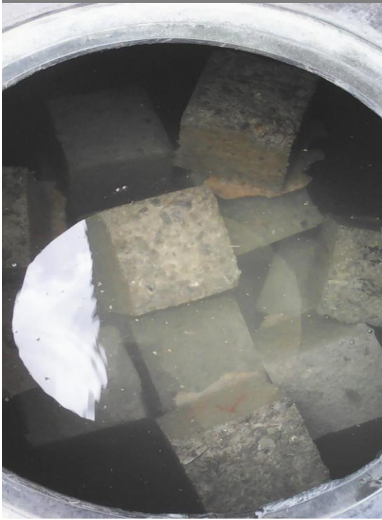
Figure 7: Curing CCH lightweight concrete in water
