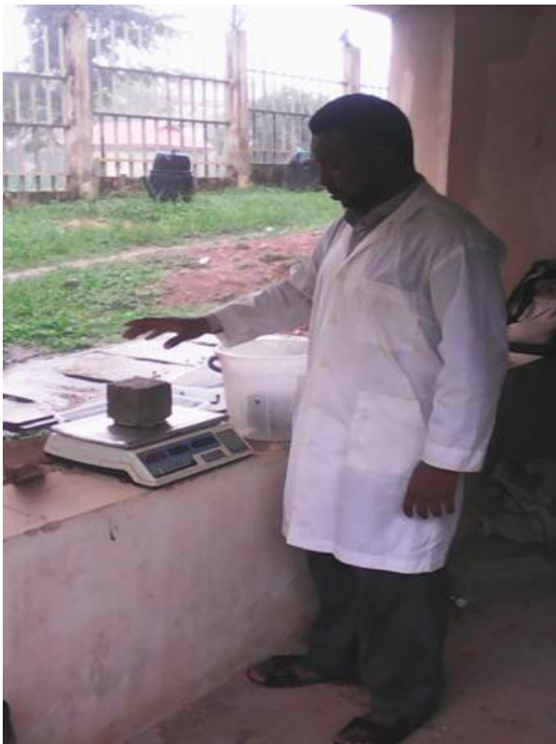
Figure 8: Weighing the CCH lightweight Concrete Cubes
