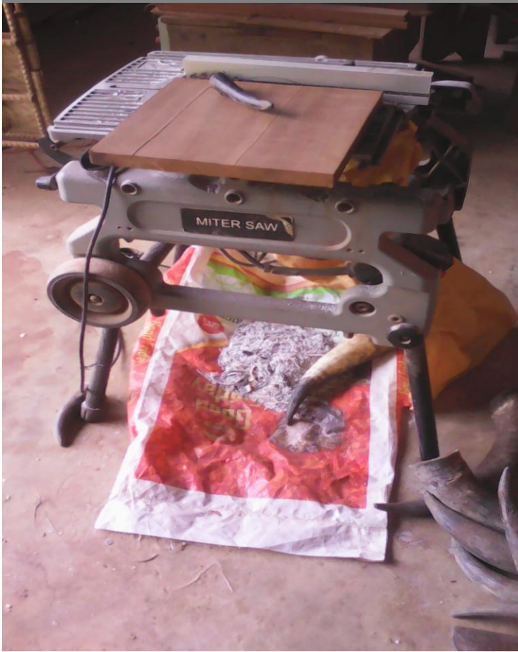
Figure 3: Cow horn shredded using Meter saw Machine
