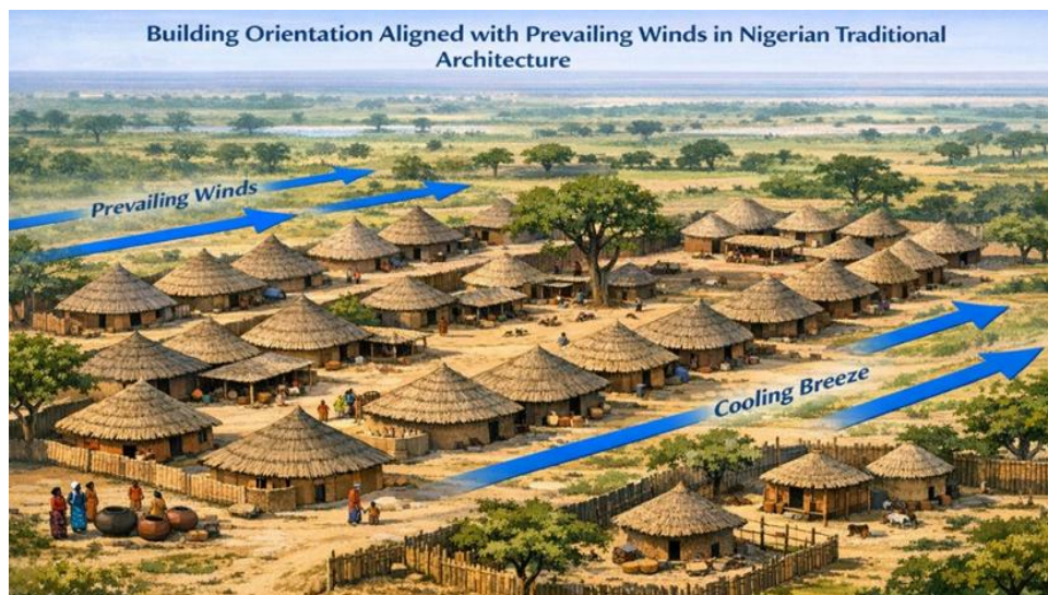
Figure 1. Building orientation aligned with prevailing winds in the Middle Belt Nigeria
