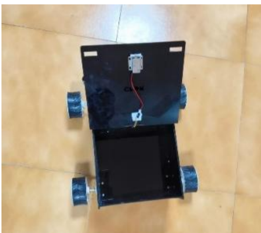
Fig 13. The solenoid compartment is unlocked only after successful verification of the user's face and associated details, ensuring secure access to the delivered package. The system uses camera-based recognition to match the
