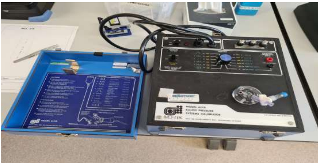
Figure 9. Biotek Fluke 601A Blood Pressure System Calibrator connected to the pressure sensing cascade. This device is capable of emulating heart pressure.
