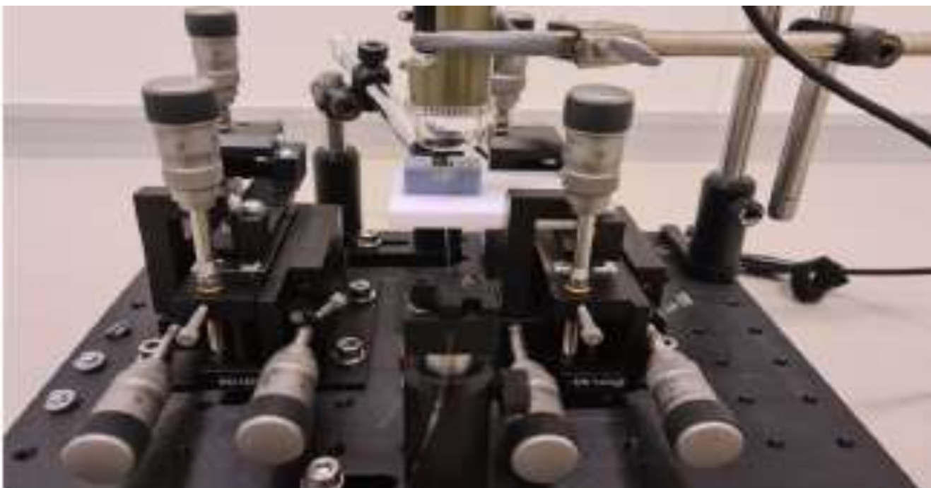
Figure 7. All FBG positions in the fibre are localized, and positioned using a 4-axis micropositioning unit in the middle of the fibre with an accuracy of 1 \mu\text{m}
