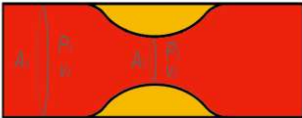
Figure 1. Bernoulli states a direct relation between cross-sectional areas A_1 and A_2 , static pressures P_1 and P_2 , and flow speeds v_1 and v_2 . If the area reduces, the static pressure reduces, while the dynamic pressure increases. This implies that a cascaded pressure sensor can be used to trace stenosis
