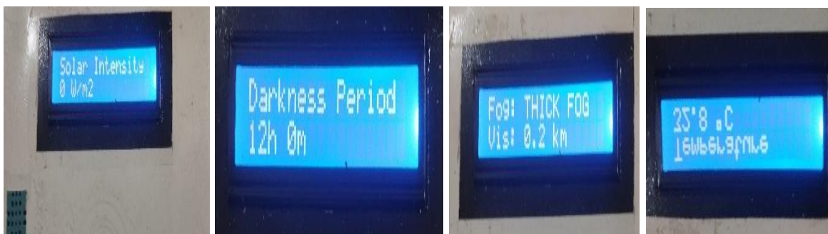
Figure 2.6: Constructed IoT Weather display showing the measured Values during Testing
