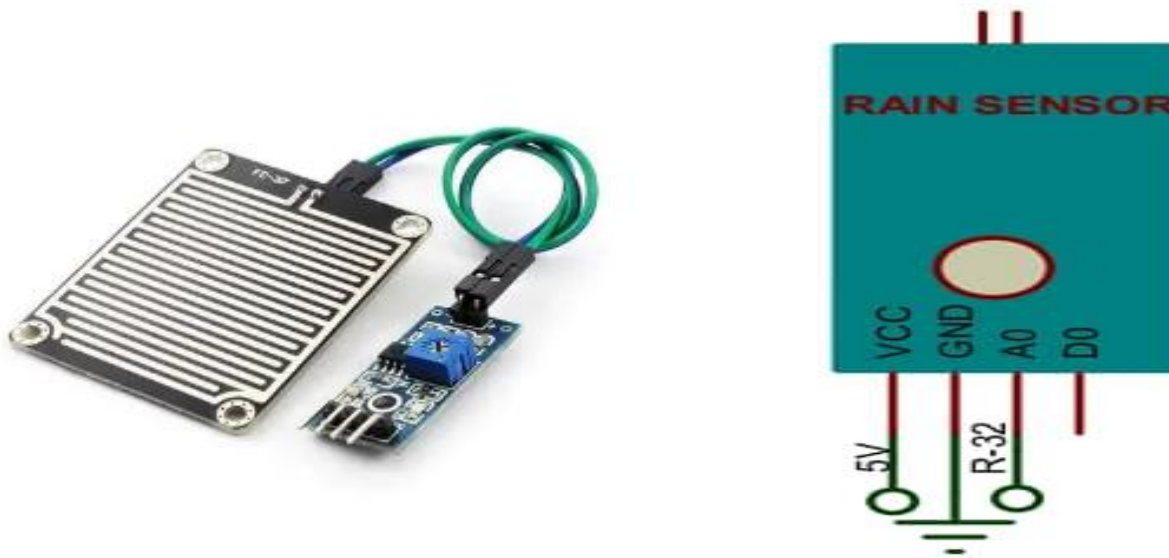
Figure 1.6: Rain sensor module and Internal Circuit
