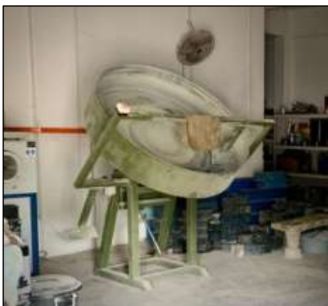
Figure 1. Disc Pelletizer Machine
