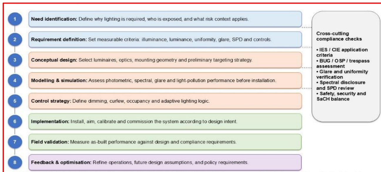
Figure 2. Performance-Based Outdoor Lighting Design Workflow
